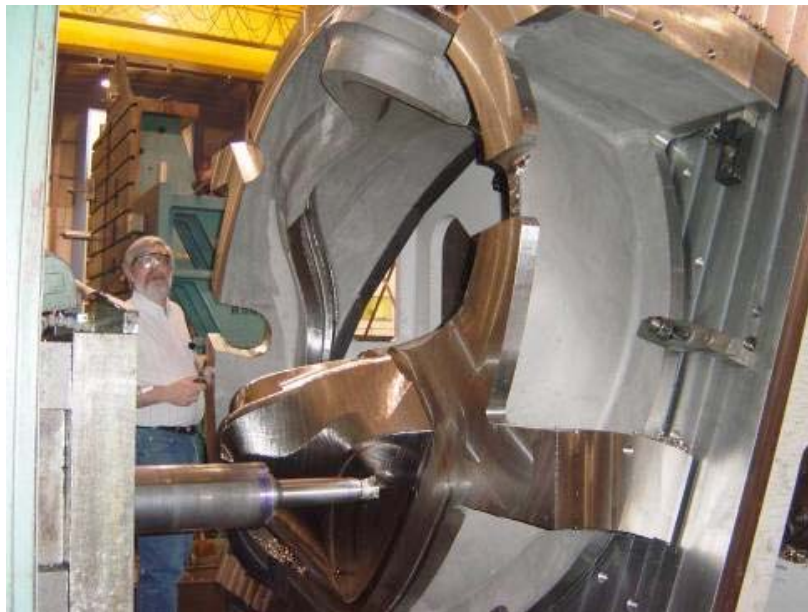
Figure 3. Machining of a NCSX Modular Coil Winding Form. Note the extended cutting tool required due to the complex geometry.
